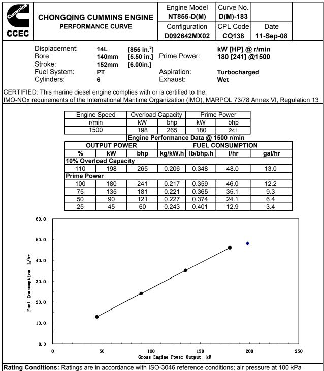
(29.61.in Hg.), air temperature 25°C (77°F), and 30% relative humidity. The fuel consumption data is based on GB252 No.0 diesel fuel (No. 2 diesel fuel in U.S.) weight at 0.85 kg/litre (7.1 lb/U.S. gal).
