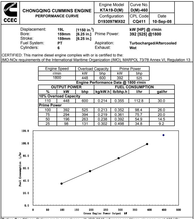
**Rating Conditions:** Ratings are in accordance with ISO-3046 reference conditions; air pressure at 100 kPa (29.61.in Hg.), air temperature 25°C (77°F), and 30% relative humidity. The fuel consumption data is based on GB252 No.0 diesel fuel (No. 2 diesel fuel in U.S.) weight at 0.85 kg/litre (7.1 lb/U.S. gal).
