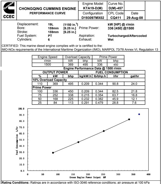
**Rating Conditions:** Ratings are in accordance with ISO-3046 reference conditions; air pressure at 100 kPa (29.61.in Hg.), air temperature 25°C (77°F), and 30% relative humidity. The fuel consumption data is based on GB252 No.0 diesel fuel (No. 2 diesel fuel in U.S.) weight at 0.85 kg/litre (7.1 lb/U.S. gal).
