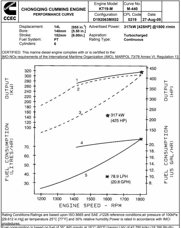
Fuel consumption is based on fuel of 35° API gravity at 16°C (60°F) having LHV of 42,780 kj/kg (18,390 Btu/lb) and weighing 838.9 g/liter (7.001 lb/U.S.gal).
